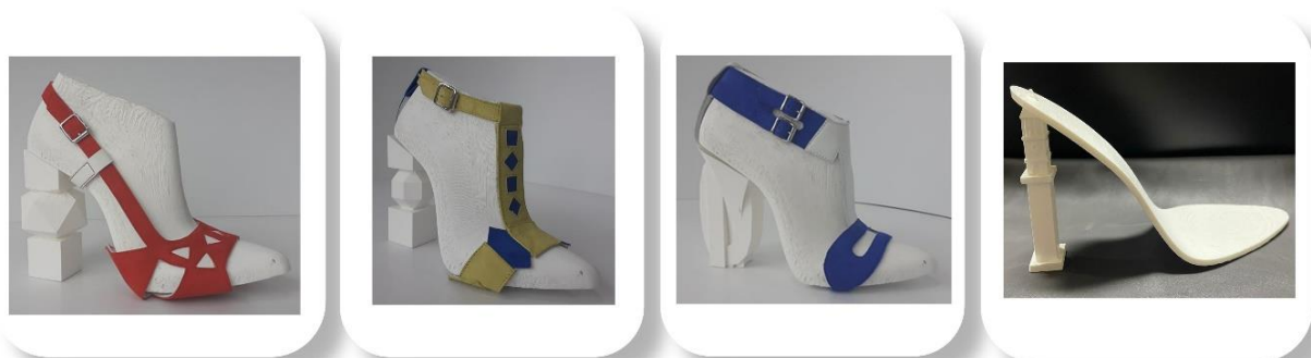
Figure 3: 3D printed shoe parts as heels and shoe last (Spahiu T., et al., 2024).
