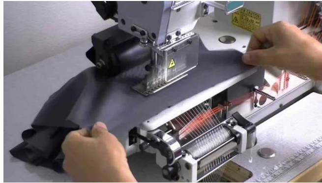
Figure 7: Shirring with the third elastic thread and a bottom metering device for elastic threads
