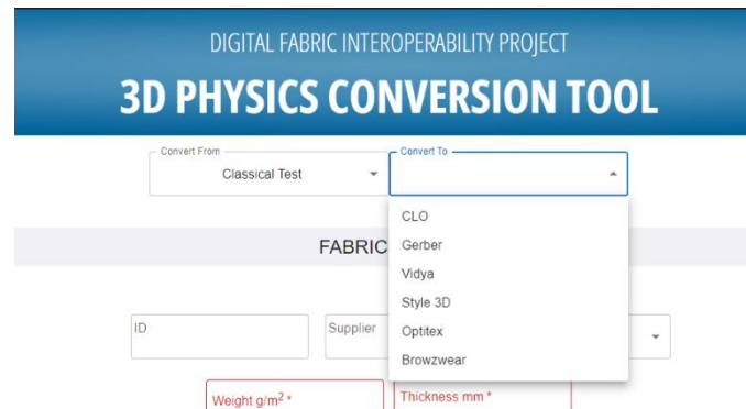
Figure 5 Web App (“3D Physics Conversion Tool”), which is developed and made available by the 3DRC to convert the results of a classic textile test to the requirements of the individual programs.
