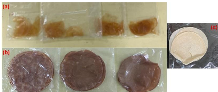
Figure 3: Photographs of PVDF films dried at different temperatures (a) 120°C, (b) 60°C, (c) 20°C
